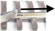
Push rail joiner back out to engage connecting track section.
