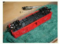
**Final Adjustments:** Turn the car upright and sit it on the bench to compare the height of the couplers to a car you already use, or to a coupler gauge such as the Kadee #205.
