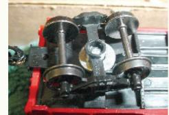
The situation becomes more difficult if you need to *lower* the car. The most effective way is to remove the nuts, and drill the hole for them a bit deeper. Reseat the nuts, apply glue, allow 5 minutes to bond, then file away the surrounding plastic material. (You may also remove material from the bolster of the truck. But this will result in a truck that probably can't be used elsewhere this is a last resort).
