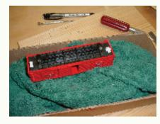
It may be helpful to secure the car using a make-shift cradle as pictured at left. Mine is just a small cardboard tray with a cloth in it which is sufficient to keep the car in place while I work on it.
