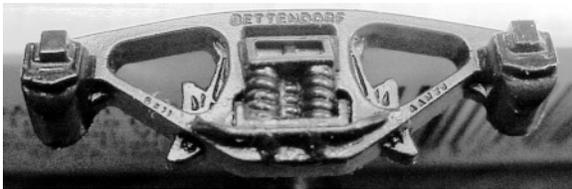
The predecessor truck was the "Bettendorf" which included 2 visible springs in front and "hot boxes" in which the axle rested and rotated in a simple hole. Appropriate for the early to mid 20th century, this was known as a "friction bearing" truck.
