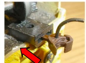
**Lower edge of end wall removed.**
