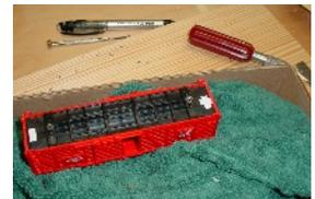
We use a 13/64th's bit to ream out the mounting socket, for a press fit of a 2/56 nut. You may use a smaller bit, then continue with a sharp hobby blade to scrape away more material. The important thing is to not make the hole too big, so the nut drops right through it. For this work, you will probably find it easier simply to hold the car with one hand, while you work with the other.
