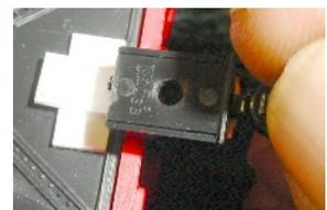
The other fix is simply to use shims from the get-go. It is a bit more time consuming but not at all complex. Simply add enough to make a platform for the coupler box, that is even with the lower edge of the end wall, as shown at left.
