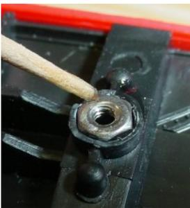
We suggest squeezing out a small drop on the tip of a toothpick, then very carefully touching the tip of the pick
