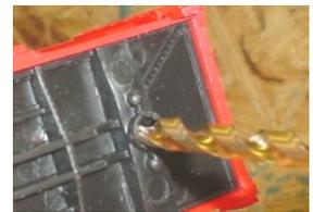
With some finger tip force, you should be able to push the nut into the hole, although it may be noticeably tilted as shown at right. Now you can drive it the rest of the way home with a flat straight edge, so that the nut is firmly seated, flat, and even with the surrounding plastic.
