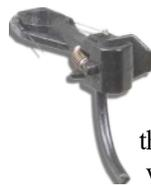
We have standardized on the Kadee because of its universal acceptance and proven operation and reliability. That brings us to two choices. The #5, with a separate spring inside the coupler box, and the #48 "whisker," (left) which relies on a thin flexible wire integrated into the coupler itself.
