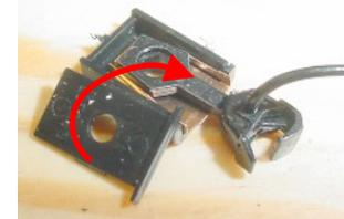
indicated by the pictures, the curved trip wire of the coupler should face toward you when you assemble the couplers. It is the closed side of the coupler box that is affixed to the car body, so the lid is in view when you pick up the car and hold it upside down.
